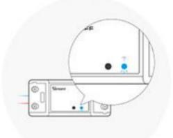
Check Wi-Fi LED indicator flashing status (Two short and one long)
