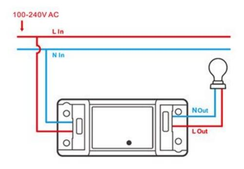
\*Please power off before wiring. To avoid electric shock hazards, do not operate any connection or contact the terminal connector while the device is powered on!
