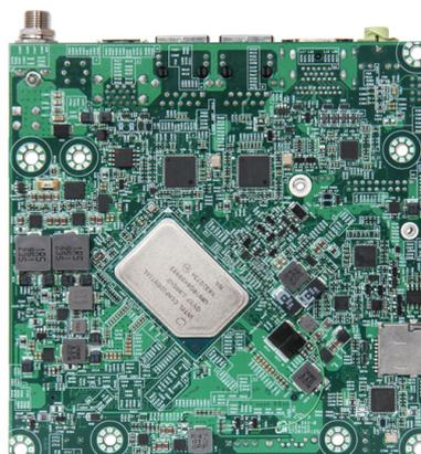
NANO-6063 is based on Intel® Atom® x6000E Series processors (formerly Elkhart Lake) integrated with Intel UHD Graphics. It supports industrial temperature range from -40°C to 85°C and can operate with TDP under 12W for fan-less applications.
