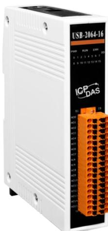
The USB-2064-16 is a 16-channel power relay output module with the USB interface. It provides a maximum 3A driving load current for variety applications. In addition, This module also provides the safety functionality to secure devices in the field. Besides, it also supports power-on configuration to customize initial state.
